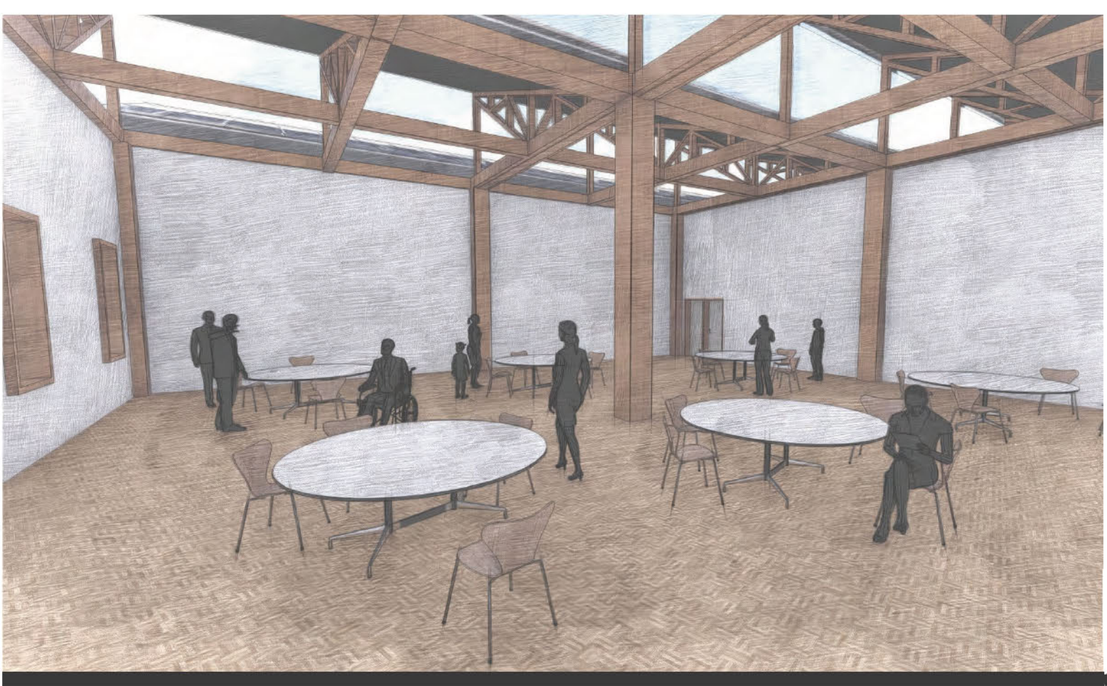
The multi-use classrooms will provide an opportunity for hands-on and visual learning experiences, within a space that highlights sustainable features such as the saw-tooth roof with skylights that allow for north lighting for an optimal work environment.
