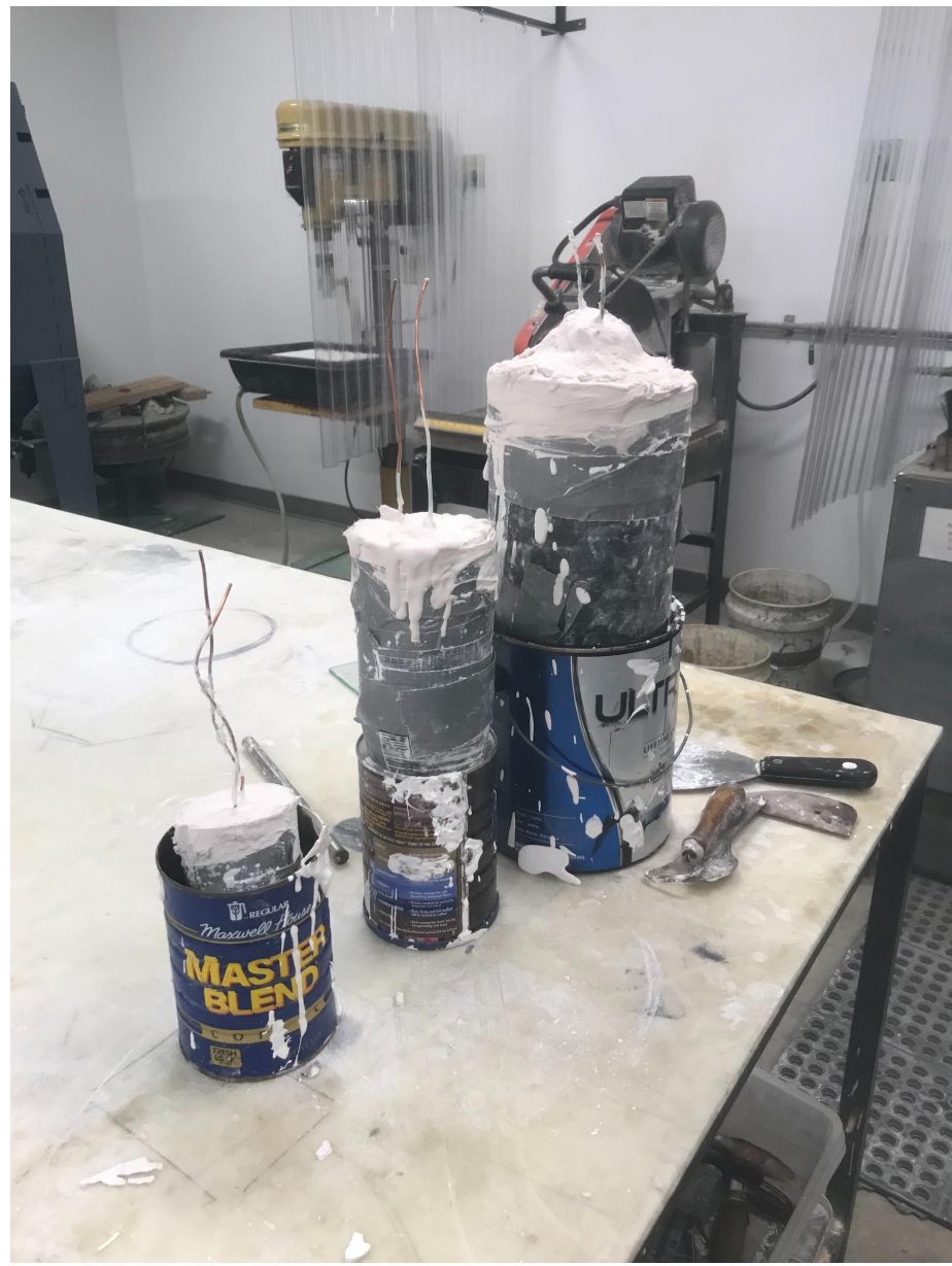
The image above demonstrates how the 3D prints were used to cast the plaster cores.
