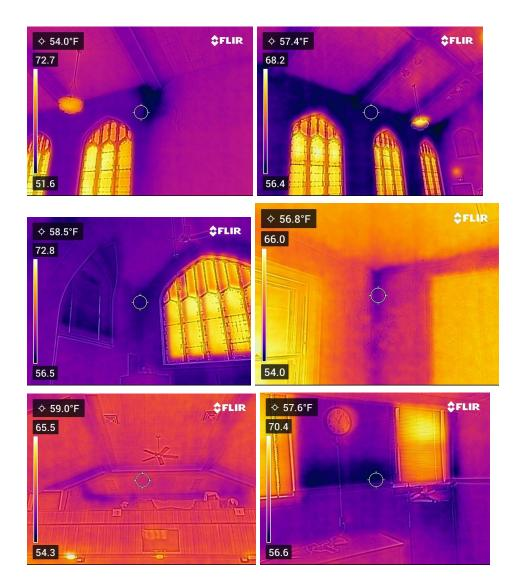
The group of images above display problems with the insulation in the building. Bad insulation is common around windows but in areas such as the one in the very first picture, it can lead to more problems. From an energy saving standpoint we recommend getting some of these spots looked at in order to save money from heating in the future.
