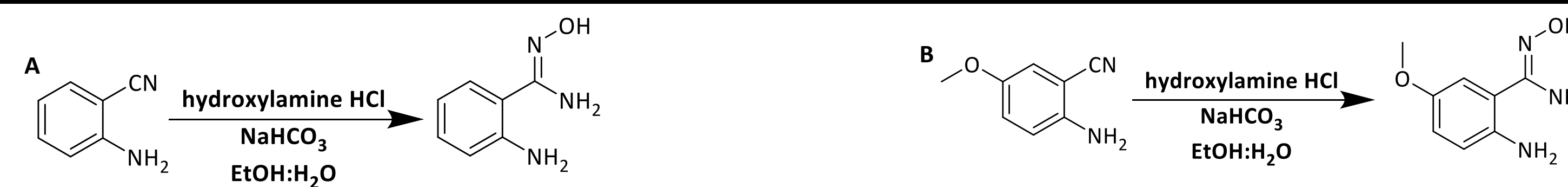
Figure 8: Reaction schemes for synthesis of (A) ABAO probe and (B) MeO-ABAO probe 7
