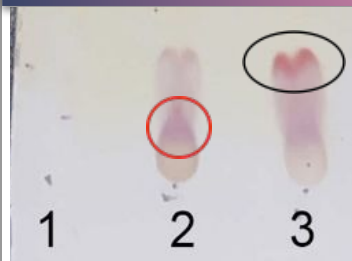
Figure 1. TLC of mitoNEET (1), mitoNEET+cysteine (2) and cysteine (3). The black circle shows spot containing cysteine. The red circle shows new spot that appeared when mitoNEET and cysteine were present.
